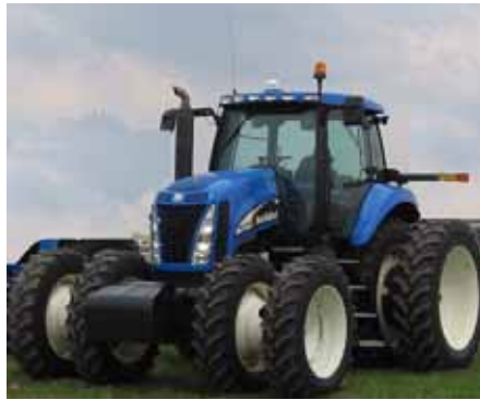
Figure A-6. Machine ballasted with full set of front suitcase weights and rear wheel weights. Wide stance with duals front and rear for stability and traction.
