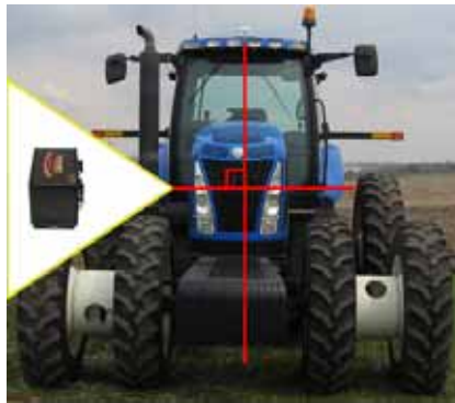
Figure A-4. Automated steering controller mounted in the front right corner of vehicle cab floor. (Level surface perpendicular to plumb line of the GPS antenna.)
