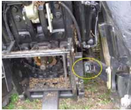
Figure A-7. Vehicle 3-point sway block set tight and spaced evenly on both sides.
